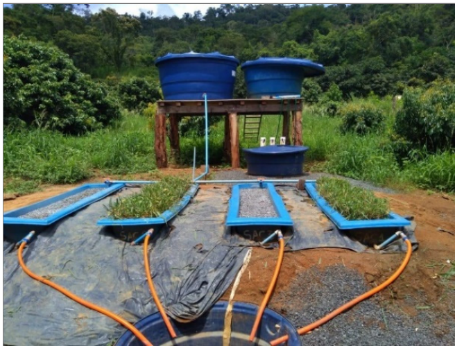
Fig. 5. CWS cultivated with Tangola grass immediately after cutting
