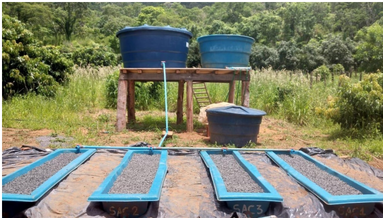
Fig. 1. Experimental bench showing the reservoirs and CWS filled with gravel
